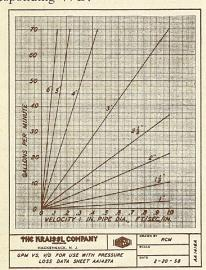
Then with Chart No. AA-1427A use this computed V/D and project to the curve of the applicable viscosity. This point can then be projected to the pressure drop axis and the data read off directly.
